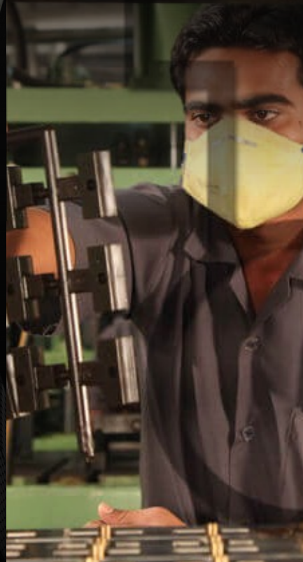
Wax Injection & Pattern Assembly
